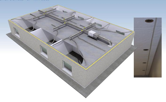
With the use of a high pressure area to low pressure area, the air in the room is continuously mixed, creating even temperatures from floor to ceiling.
